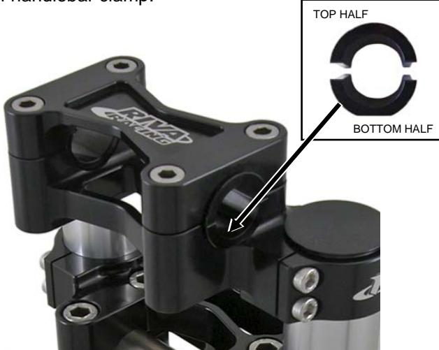
**NOTE:** Thoroughly clean bars, billet spacers and handlebar clamping surfaces with a non-residual cleaner. Apply red Loctite to handlebar clamp bolts. **Torque bolts evenly to 14 ft•lb / 20 N•m.**
