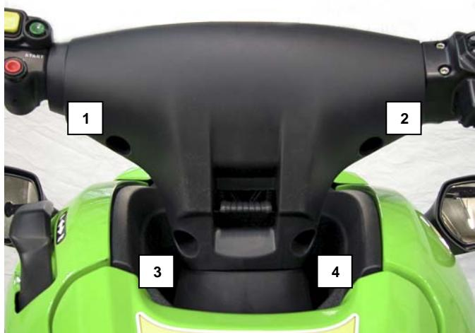
Remove handlebar pad foam.
